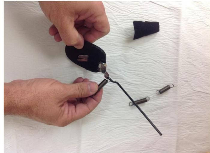
Secure the opposite eye hole of the spring to the hook on the base plate.
