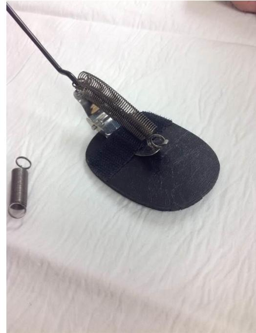
Press the two springs together to overlap the coils. Overlapping the coils helps to minimize the bulky appearance of the springs sticking out above the base plate that can occur if they are not pressed together.
